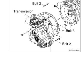
③ Using a moving truck slowly pull out transmission assembly to the front.
